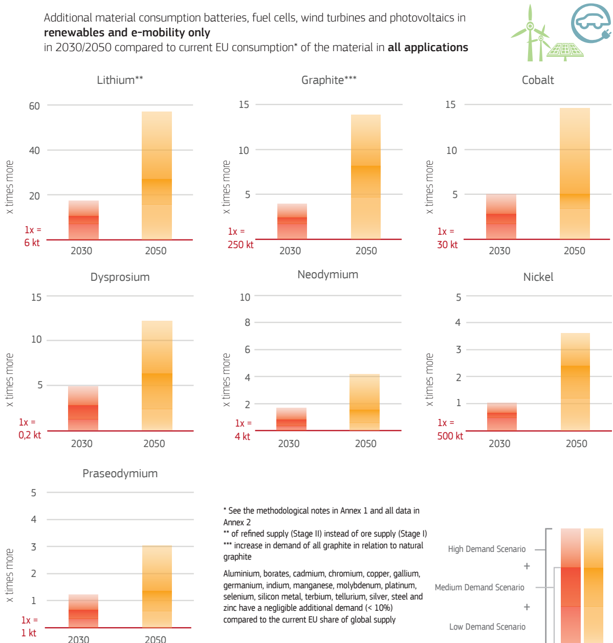
Figure 1. Combined critical raw materials use in different technologies in the EU in 2030 and 2050
